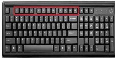
**Use:** A function key is a key on a computer or terminal keyboard that can be programmed to cause the operating system or an application program to perform certain actions, a form of soft key.
