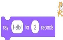
The block displays a speech bubble with the text specified for the sprite executing it, which appears on the screen for the specified number of seconds.
