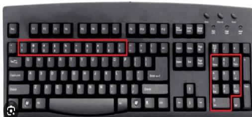
**Use:** input numerical values into a computer or other device and can also be used for other functions such as navigating through menus and entering special characters when combined with the Shift or Alt keys.
