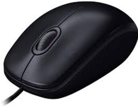
A mouse is a small device that a computer user pushes across a desk surface in order to point to a place on a display screen and to select one or more actions to take from that position.
