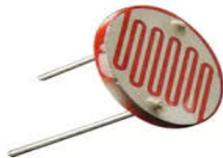
**LDR**, also known as Photo resistor Means light dependent resistors (LDR), are light sensitive devices most often used to indicate the presence or absence of light, or to measure the light intensity.
