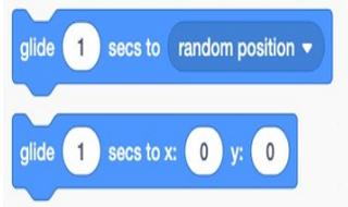
This is used to move the sprite, at a steady pace, to the chosen x and y coordinates in the mentioned time in the block, in the decided time, in a gliding movement.
