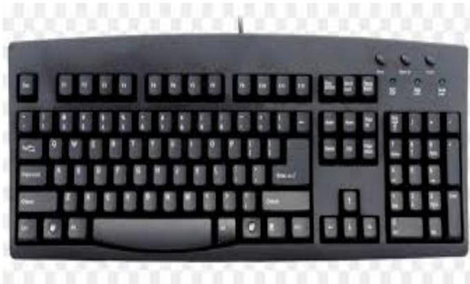
A **keyboard** is one of the primary input devices used with a computer. Like an electric typewriter, a keyboard is composed of buttons to create letters, numbers, and symbols, and perform additional functions.
